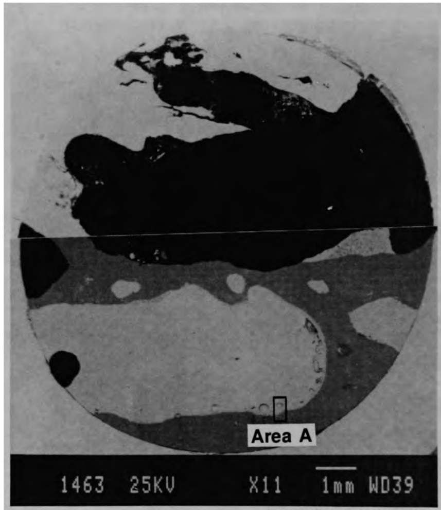
Figure E-43. Backscattered electron image of interfaces between metallic inclusions (K09-P2-D1).
