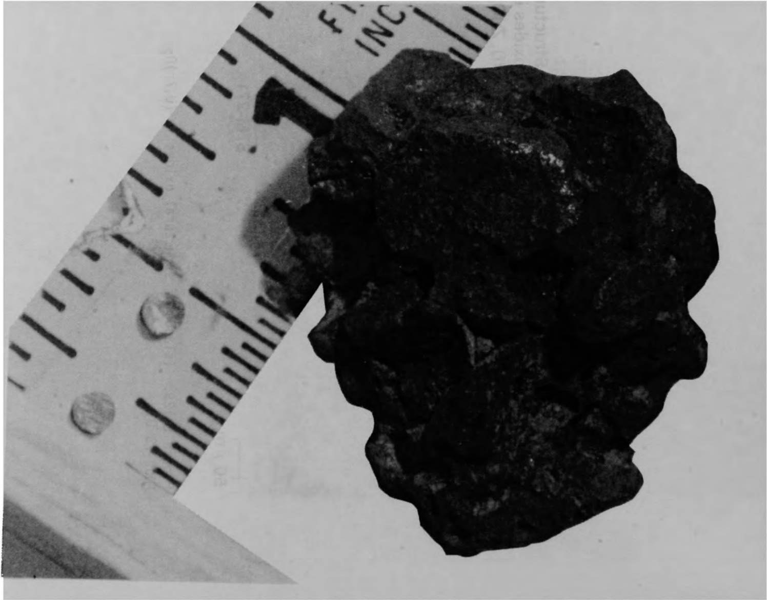
Figure E-130. Overview of ceramic sample K09-P3-F from the consolidated core region
