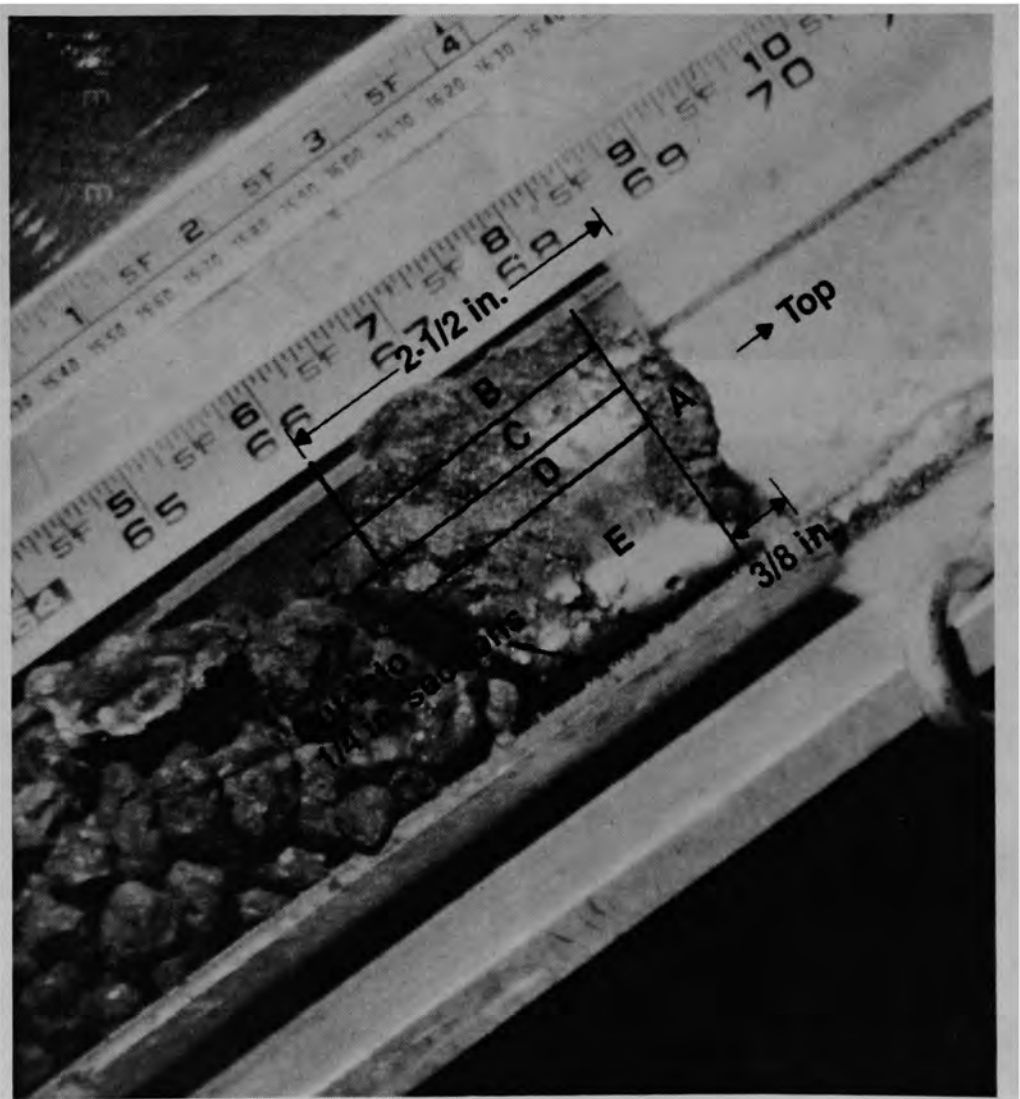
Figure E-41. Sectioning diagram for upper crust sample K09-P2.
