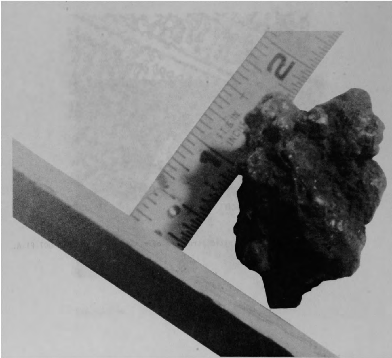
Figure E-86. Overview of metallic sample 007-P6 from the consolidated core region.
