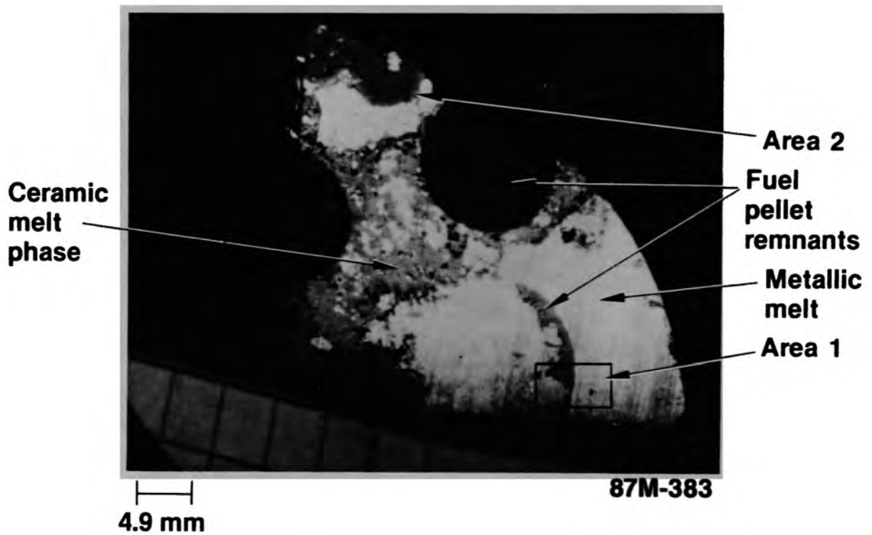
Figure E-12. As-polished transverse section D08-P2-A2.
