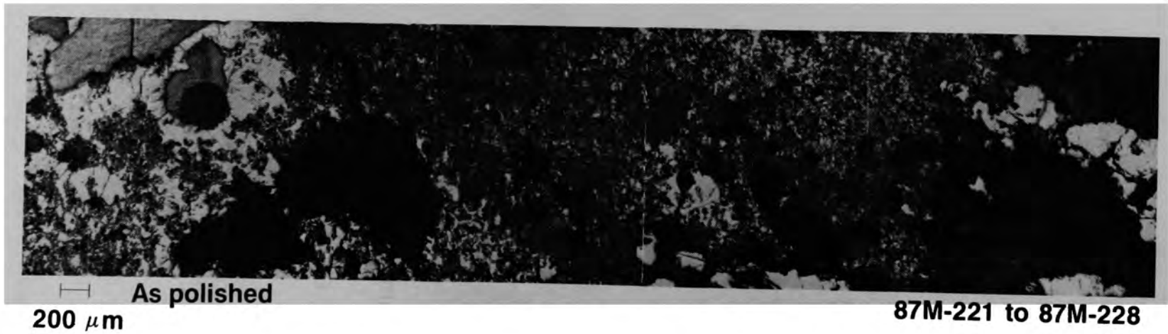
Figure E-140. Structural oxides around pores in (\text{UZr})\text{O}_2 matrix.
