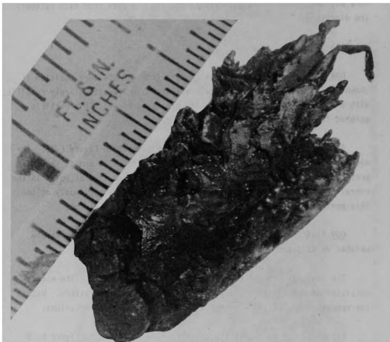
Figure E-74. Overview of metallic sample D04-P2-A from the consolidated core region.
