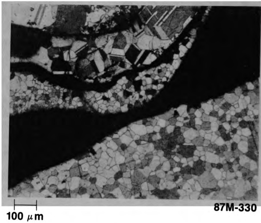
Figure E-76. Previously molten Ag-In-Cd alloy.
