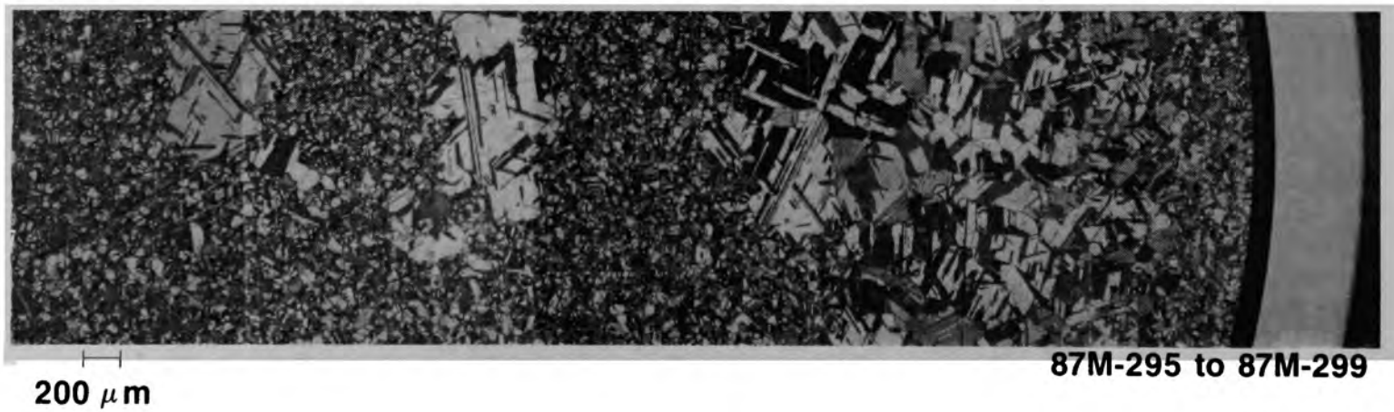
Figure E-196. Possible melting of Ag-In-Cd alloy.
