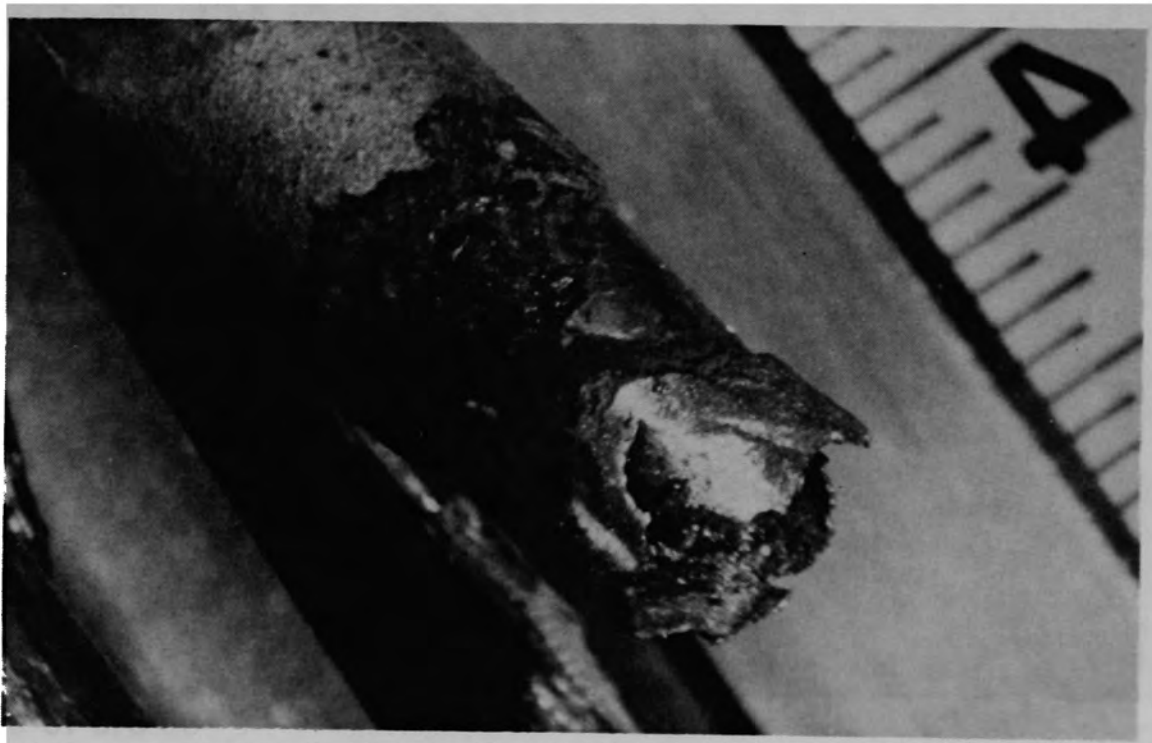
Figure C-16. Melted material at tip of rod stub.
