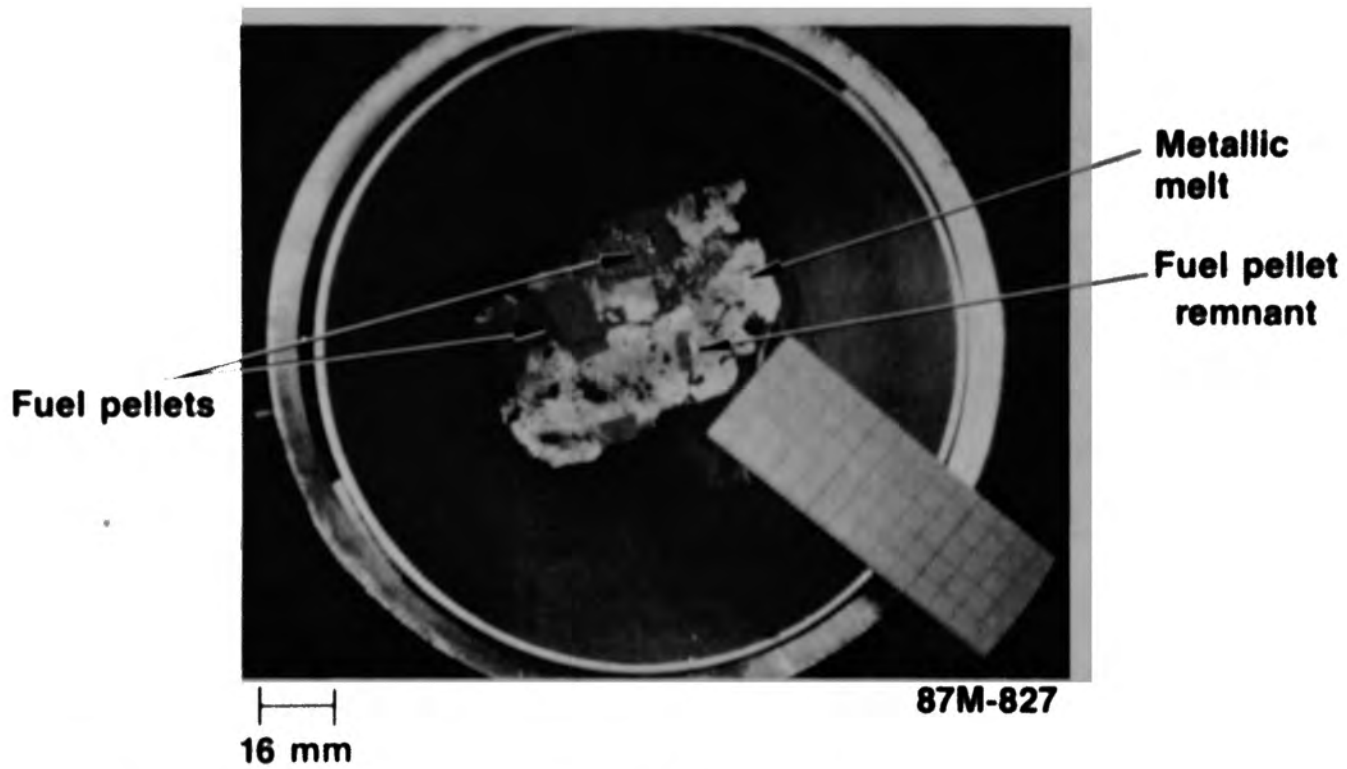
Figure E-5. Longitudinal cross section D08-P1-D from lower crust.
