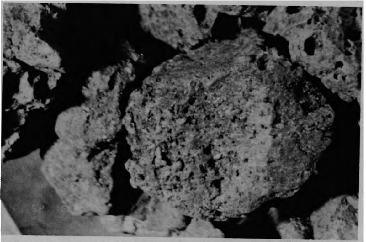
Figure C-11. Ceramic particles in K09 core bore.
