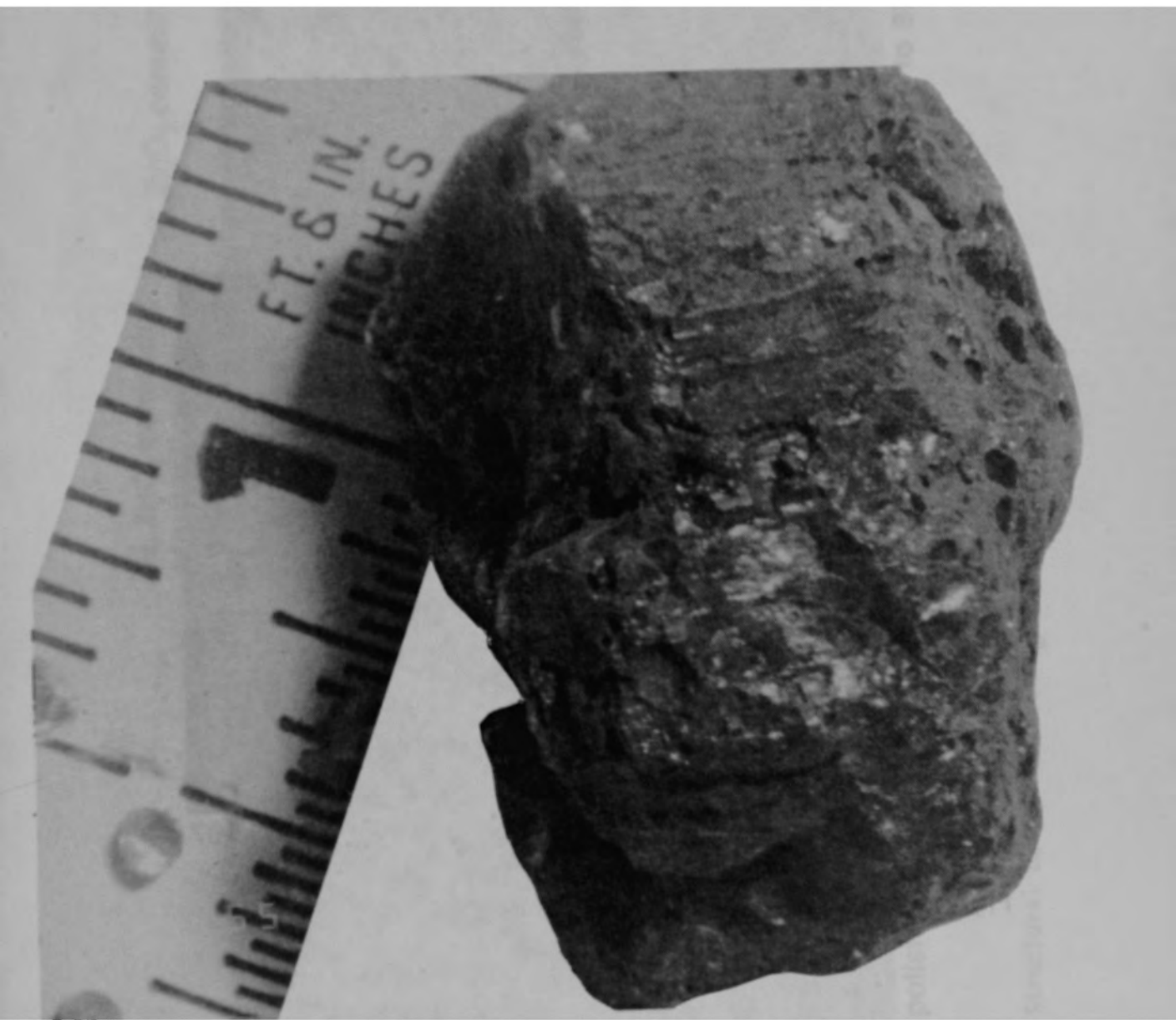
Figure E-93. Overview of ceramic sample D08-P4-A from the consolidated core region.
